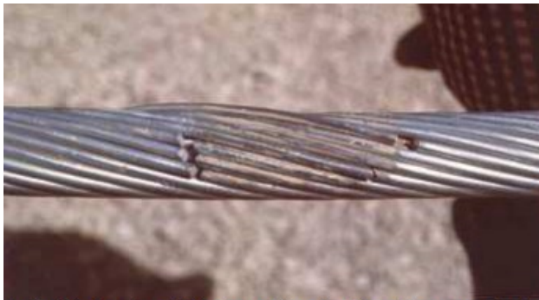
typical broken strand due to aeolian vibration after removal of suspension clamp.
