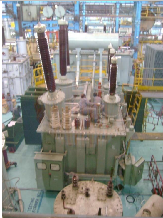
Photo 6: 50 MVA 220/132 kV Transformer
