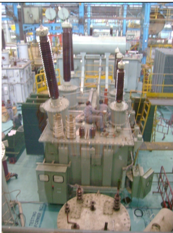
Photo 6: 50 MVA 220/132 kV Transformer
